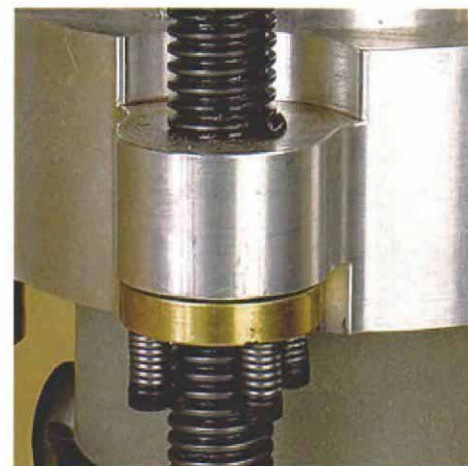
Meaty parts. The two ProLift models incorporate a heavy drive screw. A spring-loaded nut eliminates backlash.
