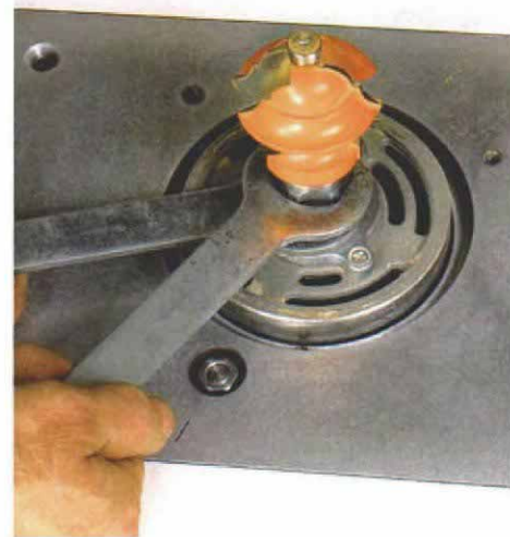
Above-the-table bit changes. Both ProLift models let you raise the router collet above the table, so bits can be changed from on top.
