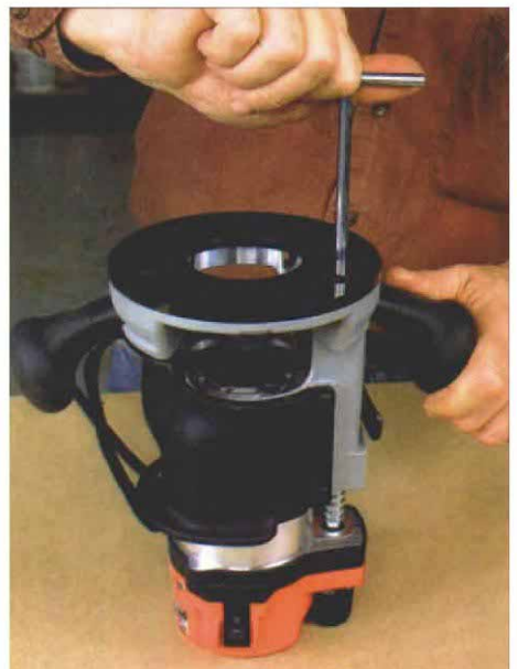
Adjustment from above. Milwaukee's new router allows you to adjust the bit height simply by using a T-wrench (supplied).
