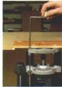
Raising (or lowering) the Raizer. The Router Raizer, like the other lifts here, uses a simple crank to adjust the bit.
