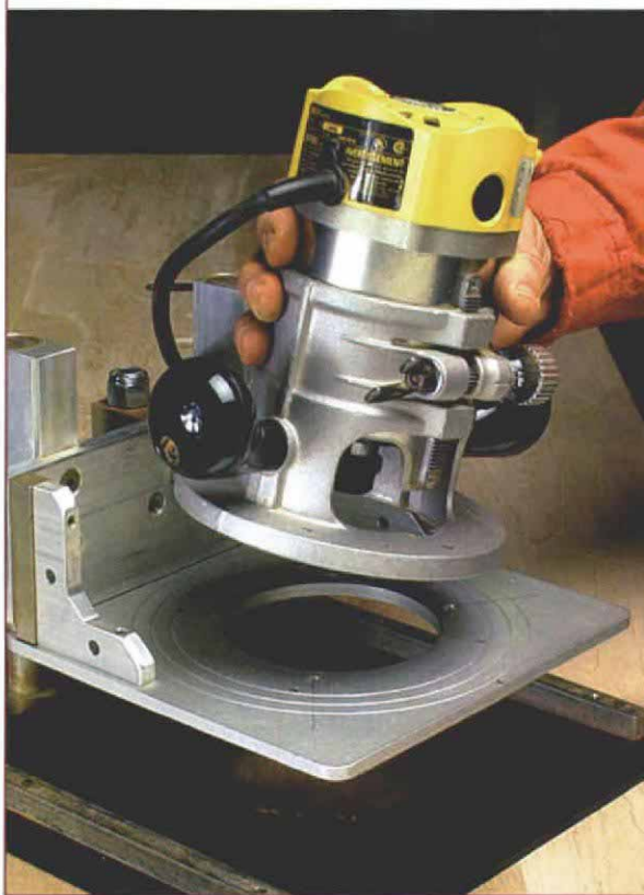
The router base mounts directly to the lift's carriage. That allows the Rout-R-Lift to accept both fixed-base and plunge routers.
