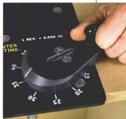
Get cranking. Each full turn of the Rout-R-Lift crank raises or lowers the bit 0.050 in. With the aid of the index marks, movements in increments as little as 0.002 in. to 0.003 in. are possible.
