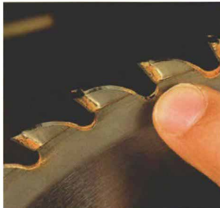
Pitch is a problem. A heavy buildup of pitch on sawblade teeth can lead to poor cutting and shorter blade life.
