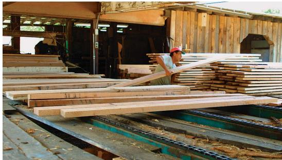
Planks from one tree go their separate ways. After being cut to length, the boards are stacked based on their length and thickness, then sent off to be kiln-dried. Even in this small sawmill, it is rare for all of the boards from a tree to end up in a single stack.
