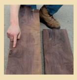
Check both sides of a board. Because small knots may not pass through a board, check both sides when looking for distinguishing marks.
