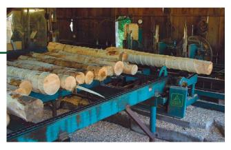
One log among many. After being debarked, logs from the same species are run through the sawmill, where the operator determines the thickness of the boards.
