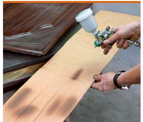
Before spraying a shading finish tinted with color, use a scrap of cardboard to set the size of your spray pattern.
