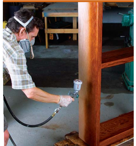
With a touch-up gun you can apply stains fast and evenly. Here, Jewitt uses the gravity-feed touch-up gun with a plastic cup to spray a water-based dye stain on an oak bookcase.
