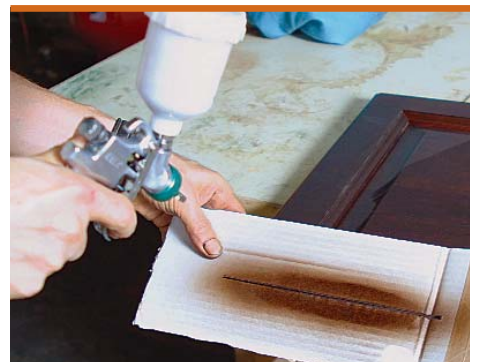
A mask makes a cleaner touch-up repair. A piece of posterboard with a sawkerf cut through it limits the amount of stain and finish applied to an edge on which the color has been rubbed through and removed.
