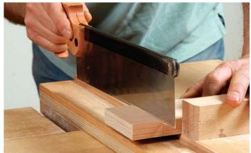
**Let the saw do the work.** There is no need to put any downward pressure on the saw. Its own weight is enough. The teeth will cut without any resistance or catching.
