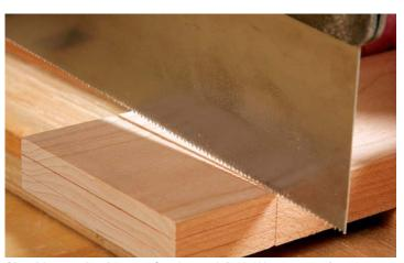
**Shoulder tracks the saw.** Set the teeth in the V-groove, against the shoulder. Lower the blade until it rests in the groove across the board's entire width before you begin to cut.
