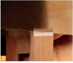
**Start on the far edge.** Align the cut with your thumb (1). Without putting any weight on the saw, gently push it forward. It's easier to get just a few teeth started straight at the back edge than to get a straight start across the board's entire thickness. Lower the back of the saw as you cut deeper (2). After reaching the front edge, bring the saw horizontal (3) and cut down to depth.
