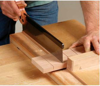
**Here's the drill for shoulders.** Use a saw hook and your off hand to keep the board still. To get used to cutting down to a horizontal line, mark the depth on both edges.
