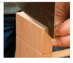
Work down the near edge. Angle the saw up and cut down the layout line closest to you.
