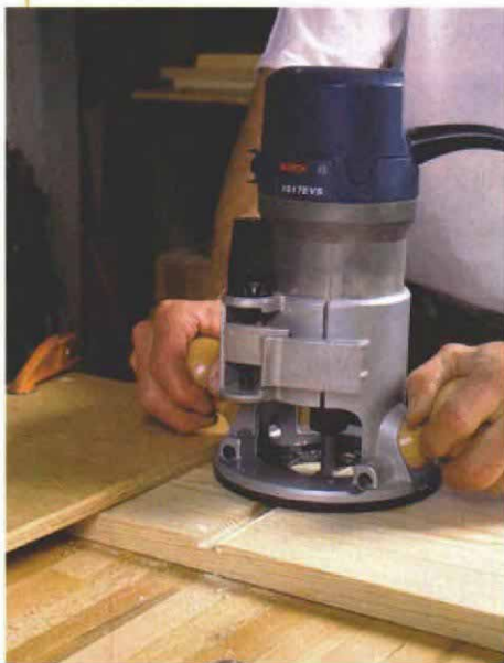
No need for a dado blade. A router guided by a straightedge clamped to the workpiece (left) cuts a neater dado than a dado blade and with less danger.
