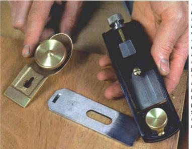
One finely made plane. The Lie-Nielsen version is a step up in the evolution of the original Stanley design. All blade and throat adjustments function precisely. The well-machined bed was the largest of all the tools reviewed, providing good support for the blade and eliminating chatter.
