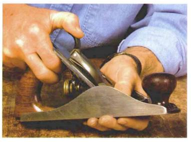
Secure the blade tightly. Planing with the tool held at an angle puts lateral pressure on the blade and can shift it out of alignment.
