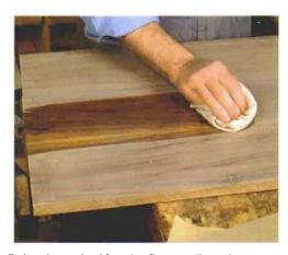
Raise the grain. After the first sanding grit, wet the surface with a damp rag and let it dry before continuing through the grits to 220.
