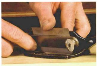
Place the tool on a flat surface. Loosen the thumbscrews and let the blade drop down level with the sole. Then tighten the screws while keeping the blade in contact with the surface.
