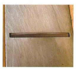
A slightly crowned plane blade won't dig in at the corners. Grind and hone a gentle curve across the entire width of the blade, with the comers about 1/64 in, back from the center.
