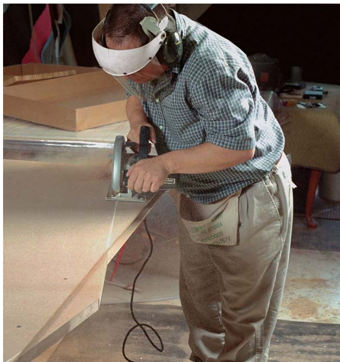
Cut the skins and frame to rough shape. After snapping a chalkline to the outside miters, the author uses a circular saw to remove much of the waste.
