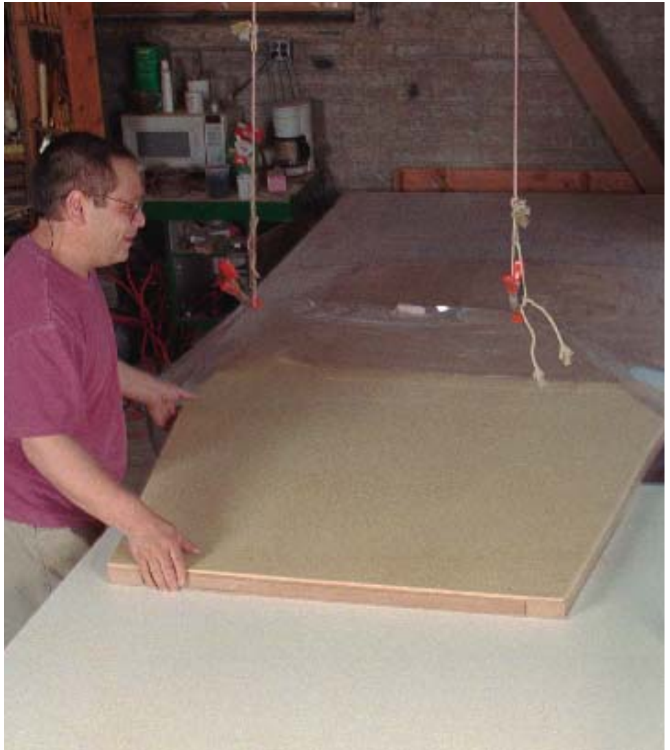
It doesn't take a lot of pressure. The honeycomb core requires only about half of the clamping pressure as that used for gluing up veneer.
