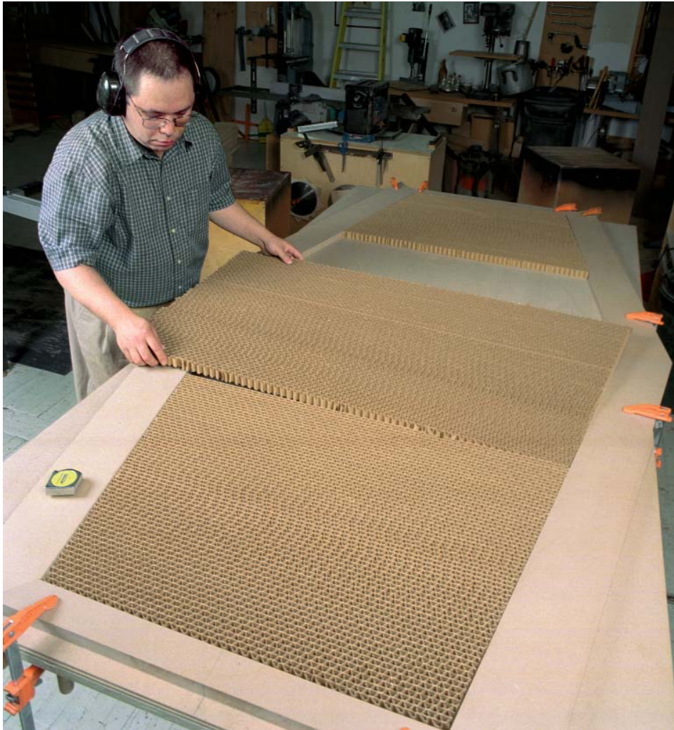
Dry-fit the core. The cardboard honeycomb, purchased in 2-ft. by 4-ft. pieces, is cut on the table-saw and fitted within the MDF frame.
