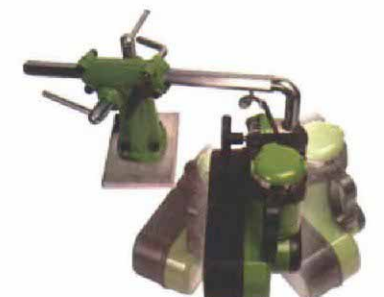
A power feeder is adjusted with a slight toe-in to keep stock from drifting away from the cutterhead.
