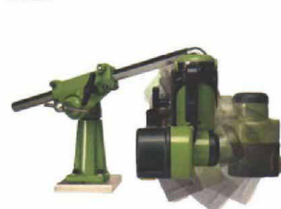
A power feeder can be set up to hold stock against a fence or to press it down against a table.
