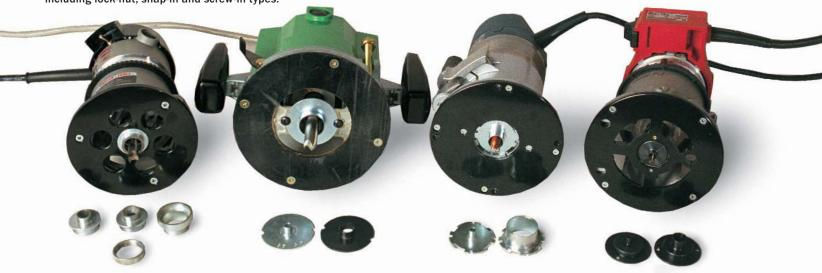
The industry standard. The Porter-Cable screw-in lock-nut system that works in all 13/16-in. subbase openings is used by many other router companies.
