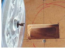
Lessen the rigors of cutting a mortise. A simple template clamped to a workpiece or a door will make cutting mortises easy with a collar.
