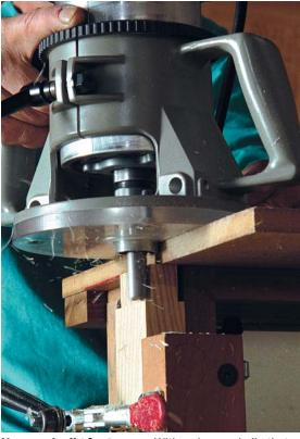
You need a jig for tenons. With a shopmade jig that will clamp the work vertically, a collar can be used to cut cheeks and shoulders of tenons at the same time.
