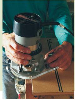
An offset subbase is a good idea. An offset subbase will help steady a router with a collar attached. You can correct for any lack of concentricity in the collar by keeping the same edge of the collar against the template. Do this by drawing a line on the template and guiding the subbase handle along that line.
