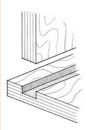
A straight pathway. There is probably no better way to cut cross-grain dadoes than using a collar. Dadoes deeper than 1/8 in. can be cut in a series of passes. Grooves that run with the grain are cut the same way.
