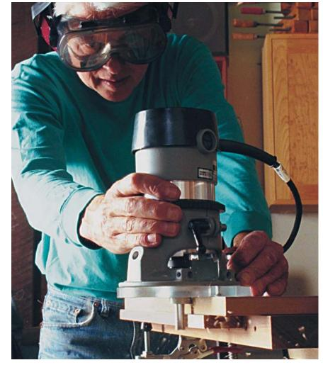
**Collars have the** edge. A collar and a perfectly straight, simple template can help a straight or spiral bit put a finished edge on long grain or end grain.
