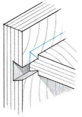
Sliding dovetails are a breeze. Using a collar and template is a slick way to cut the slot for a sliding dovetail. The same setup can be used to cut out some of the waste with a smaller straight bit before cutting the dovetail.
