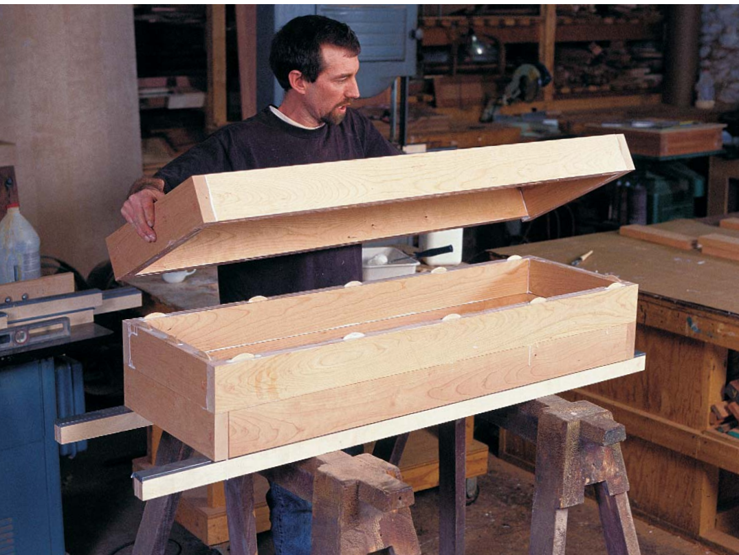
A race against curing glue. The cabinet must be glued up in one swift process. Four-board boxes are biscuited, coated in white glue, then set onto similar assemblies.
