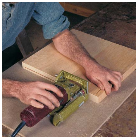
Plunge-cut the groove. To cut a groove, the biscuit machine slides like a router along the edge of the divider.
