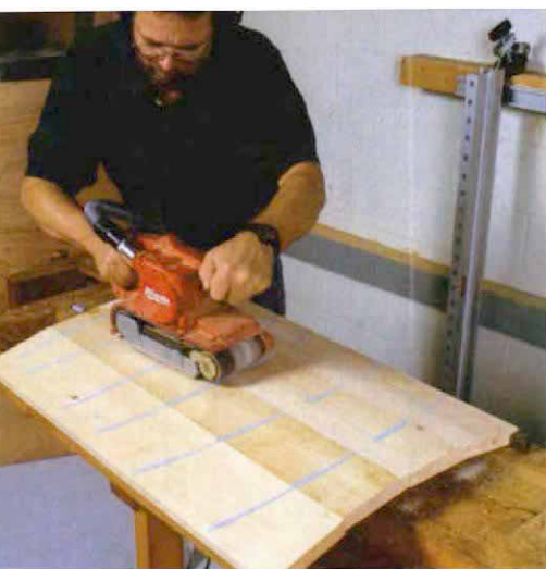
Rounding the gluelines. Horizontal chalklines stripe the surface, and only the highest spots—the gluelines—are sanded in vertical stripes until the curve nears its final shape.
