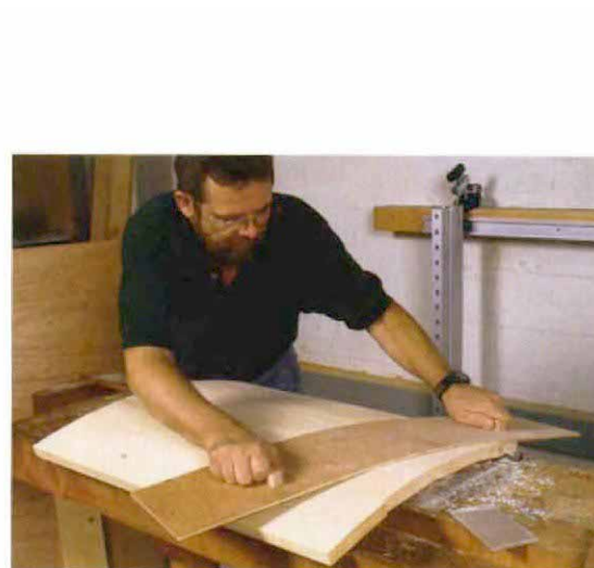
Pliable sanding block. The author glues sandpaper to \frac{1}{4} -in. plywood, which bends and slides smoothly over the surface, keeping a curve in line.
