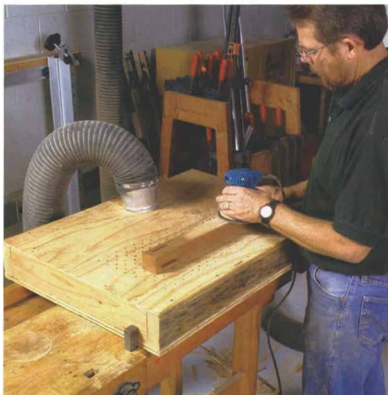
A downdraft table keeps it clean. The author's sanding table is just a box drilled with holes to suck the dust away. This simple box, made of plywood and 2x4s, hooks up to a dust-collection system or shop vacuum.
