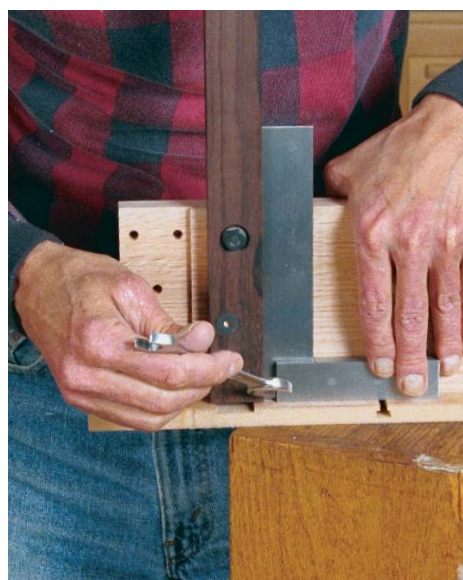
Square the fence to the platform. Tighten the two fence-mounting screws to lock the position. A slightly oversized hole allows the fence to be positioned at exactly 90°.
