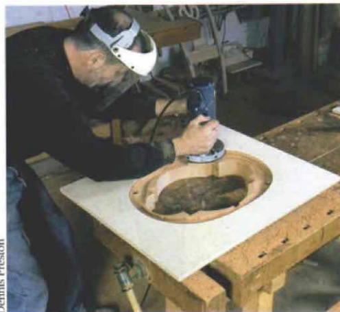
A router makes fast work of the seat rabbet. Use a full-sized oval pattern to establish the layout line.
