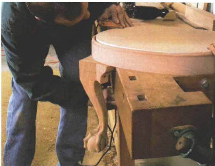
Temporary fixing. With the ball and claw complete, prepare to carve the knee by dry-fitting the leg to the frame. Use screws through the knee blocks to hold the leg in place.
