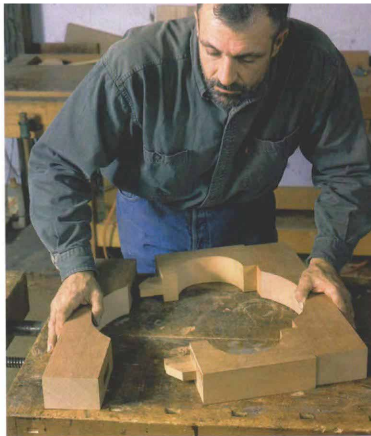
Assemble the frame. The bulk of the frame has been reduced by bandsawing arc-shaped segments prior to assembly.
