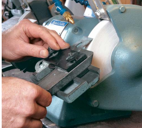
This accessory enhances safety and consistency. A heavy-duty grinding attachment designed for the Baldor No. 7306 secures the blade as you slide it in a steady path across the wheel.
