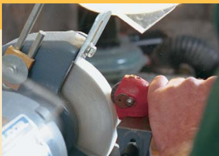
Simple steel (or “star”) wheel dressers sell for about $15. The wheels eventually wear out but can be replaced.
