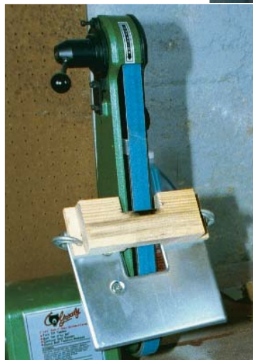
Customize the belt sander's tool rest for better performance. A block of wood, notched and back-beveled to clear the sanding belt, makes this machine more useful for a variety of blades.
