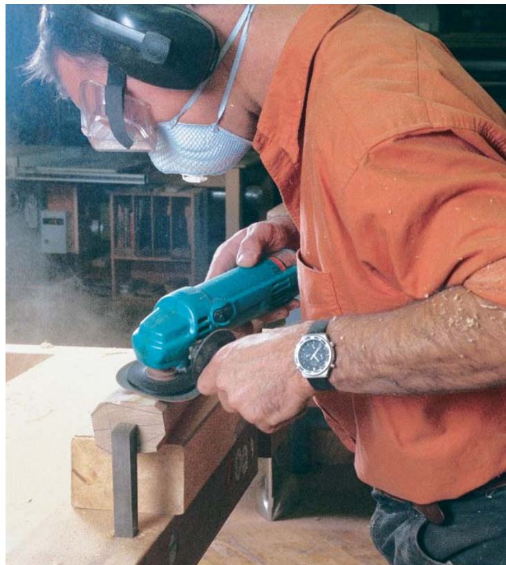
Shape the facets with an angle grinder. A 24-grit sanding disc removes material quickly. Use long, fluid motions and take light passes.
