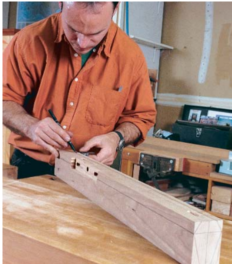
Lay out the bedposts. The six-sided shape is drawn on the end grain first, then the lines are carried over onto the faces.
