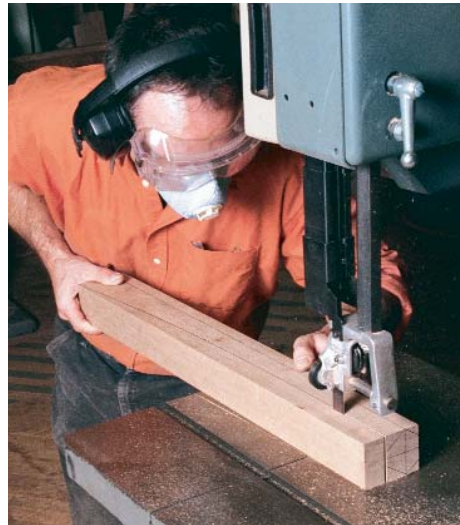
Cut the outside curve first. Bandsaw close to the line.
