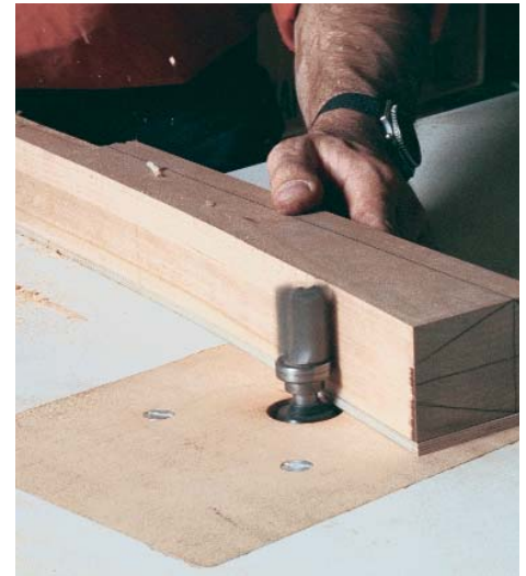
Attach the template to the post. Clean up using a router and pattern-cutting bit.
