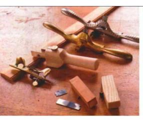
Beading tool. All beading tools work with a scratching action. Front to back: two shopmade scratch stocks, Woodcraft's bronze beading tool, the Veritas beading tool, Lie-Nielsen's bronze beading tool and a Stanley No. 66.
