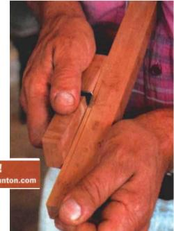
Step back and plane forward. To give the plane some bead to track on, start a plane's length in from the far end. Plane forward to the end, back up a length, then plane forward again. Continue stepping back and planing forward until you've beaded the full length. Then you can plane the entire bead to its full depth.
