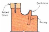
Hone and check, hone and check. As you sharpen a plane iron, stop frequently to sight down the plane (left). The iron should conform to the sole, but keep the quirk iron slightly wider than the quirk boxing (drawing above) to prevent binding. This plane reveals inlaid boxing as well as an extra fence, screwed on to improve tracking and stability.
