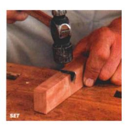
Scratch stocks are good examples of craftsman ingenuity-they are simple to make and work extremely well. A piece of hacksaw blade, bandsaw blade or similar steel makes an excellent cutter and also works as a cutter for a Stanley No. 66 beading tool.
