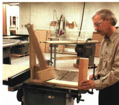
Getting whacked. Swinging a 2-ft-long, 3-lb. pendulum at the outfeed end of each fence approximates what happens in a shop when a fence gets knocked by heavy sheet goods. After whacking the fences, they were checked for parallelism. All but one fared well.
