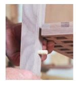
I considered several ways of attaching the grate to the legs, but settled on resting the grate on four dowels, one protruding from each leg (see the photo at left). With a ½-in. reveal between the grate and the legs and with the dowels half-hidden in notches in the underside of the grate, anyone walking up to the vanity will perceive the grate as floating.
