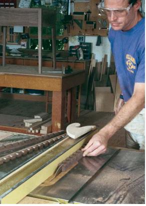
Rip the blank into notched strips. When you rip a really wide board into narrow strips, you have many chances to kick the board off square as you pass it through the saw, resulting in tapered strips that don't fit well together. You're better off ripping boards that are 3 in. or 4 in. wide.
