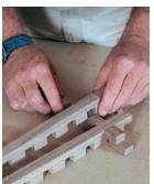
First cross-dado a long blank using a simple jig. With this jig, you'll be able to index a series of consistent dadoes across a 1-in.-thick by 3-in.- or 4-in.-wide board.
