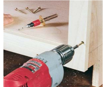
The sleeve is then removed and set aside to reveal the driver.
