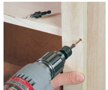
With the driver in place, the drill is readied for driving screws.
