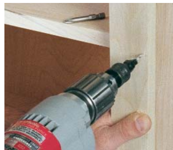
Pilot hole and counterbore are both drilled in one stroke.
