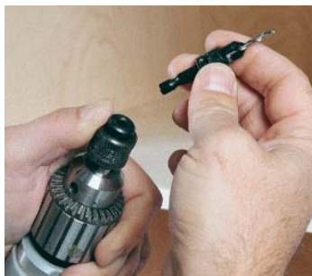
Bit locks into place with a detent on its shank.
