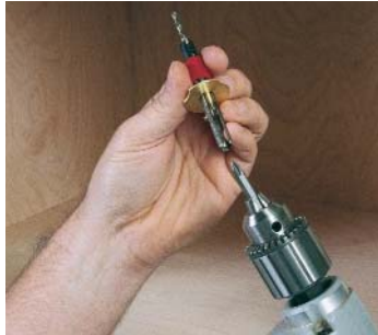
The prongs slide over the driver, which is chucked in the drill.
