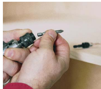
Bit is easily removed and replaced with a driver.
