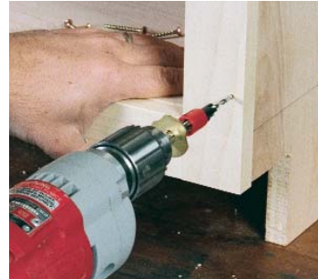
The pilot hole and counterbore are made in one easy motion.
