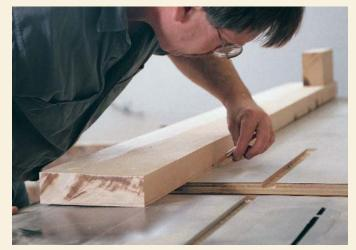
In cabinet work, I often have to scribe a flat cabinet to fit a warped wall. I flipped the concept on its head and found a way to scribe a crooked board using a flat surface for reference. Then I use the scribe marks to guide a powered hand planer and flatten one face.
