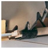
**Cutting round tenons on square stock.** Slip two pieces of PVC pipe over a spindle. Carefully rotate the spindle against the radial-arm saw's fence and a stop block while moving the cutterhead, fitted with a dado blade, to remove the waste.
