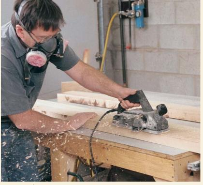
After scribing, flip the plank over, and remove waste with a power planer, paying close attention to the scribed line. Finish up using a No. 7 jointer plane. To check your progress, flip the plank over onto the outfeed table and see if it rocks.
