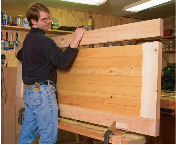
When everything is square. Work blocks clamped to a sawhorse hold the door steady while it's dry-fit. Using a polyurethane glue allows plenty of time to make sure that everything is flush, square and aligned. Just remember to mist the biscuits with water to help the glue cure properly.
