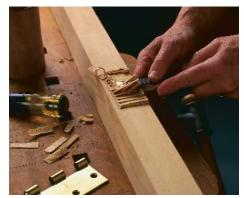
Adding detail to an unassembled frame. Work moves quickly throughout the shop when you don't have to haul a heavy door from one work area to the next. With the stile clamped securely in the bench, a series of chopping cuts and a smooth pass pares the waste away for a clean mortise that fits every time (above). To prevent tearout when boring for the lockset, drill the beveled edge first, then make two half-depth face bores (right).
