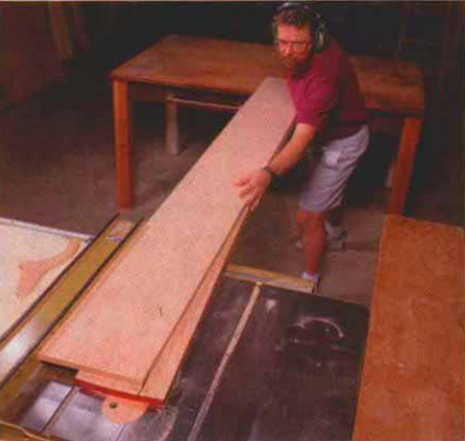
Edge-jointing without a jointer. Template registers against rip fence and guides uneven boards through a straight cut
