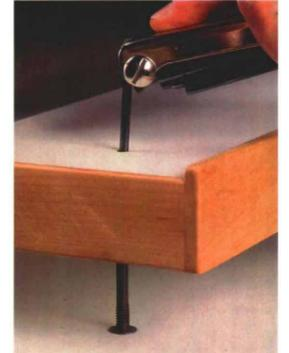
*Leveling the table*-Connector bolts screwed into threaded inserts allow precise adjustments to the height of the planer table.
