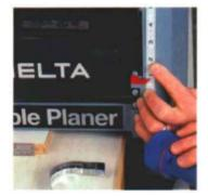
**Reset the depth scale**—To correct a <sup>3</sup>/<sub>4</sub> in. loss of cutting depth, install a new scale or reset the old one.
