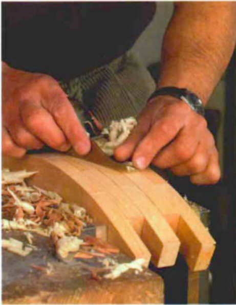
Block planes handle difficult grain. This bricklaid arch presents end grain and long grain and everything in between. For more control, use a two-handed grip, and skew the blade as it cuts.
