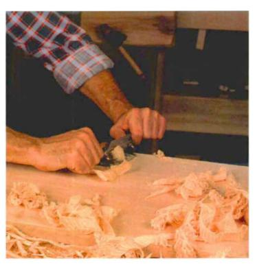
Scrape with the grain across the width of the panel from either end until you've eliminated all cross-grain planing marks.
