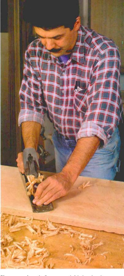
Plane across the grain. Start at one end of the board, and work to the other, planing straight across. Skewing the plane at 45° or so may help it cut better. The jointer plane's length makes it a good reference surface, and its wide iron (25% in.) allows you to make fewer passes. If the board starts to rock, tap wedges under the high corners.
