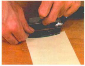
Use a piece of paper to set blade height. With a slip of paper under either the front or rear edge of the scraper sole, lower the blade until it rests on the bench. Then tighten the thumbscrews to exert pressure on the blade.
