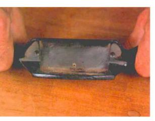
File the scraper body. Make sure the blade bed is filed flat, and file the scraper body so the retainer bar seats properly when tightened. This will help eliminate chatter and produce a better curl.
