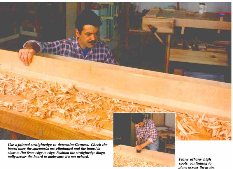
possibility of the plane blade catching the grain and lifting and breaking wood fibers. After using the jointer plane, I scrape with the grain. Because of the angle at which the cabinet scraper holds the blade, there's no chance of tearout. This lets me arrange boards for glued-up panels so they look their best, regardless of which way the grain goes. It also allows me to flatten even heavily figured wood.
