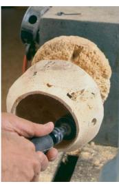
A flexible shaft will reach inside. This homemade tool (a drill chuck holding a sanding drum on the end of a flexible shaft) makes shaping and cleaning out the inside surfaces easier.
