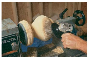
Grinding as an intermediate step—After rough-shaping with the gouge and before sanding to a final smooth shape, the author sometimes uses a grinder with 60-grit paper to remove deep pits and to refine the shape of a vessel.
