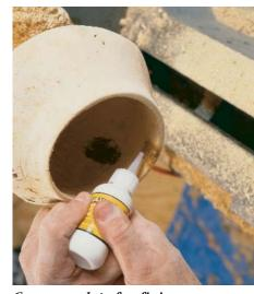
Cyanoacrylate for fixing repairs—The author prefers fast-setting Hot Stuff adhesive for its strength. He mixes mineral oil with sawdust or shavings from the turned piece to maintain a good color match and then applies the glue over that.
