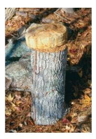
Spreading the disease-To promote fungal growth, cover the top of a log with shavings, and stack an already spalted piece of wood on top. Dampen the log with a hose. Signs of good fungal growth should appear within a few months.
