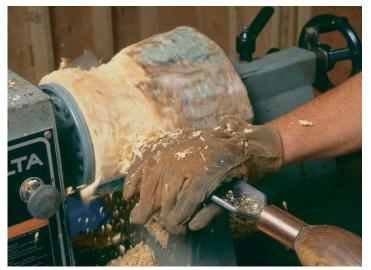
Start the lathe at a slow speed when roughing out the shape with a gouge. Soft, spongy wood cuts differently from sound lumber: It chips or breaks more than it cuts.
