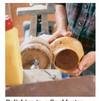
Polishing to a final luster— After several coats of mineral oil and hand-rubbed brushing lacquer applications, the author buffs each piece with tripoli polish applied to a set of heavily oiled cotton pads. He recommends an occasional coat of mineral oil to refresh an aging finish.
