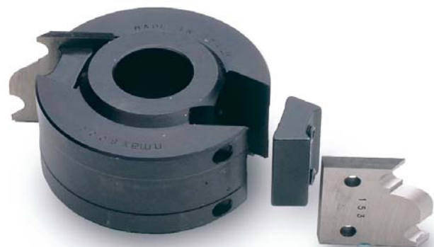
Wedge-shaped gibs hold the knives in place. A pair of pins holds each knife to the cutterhead if the gib ever loosens.
