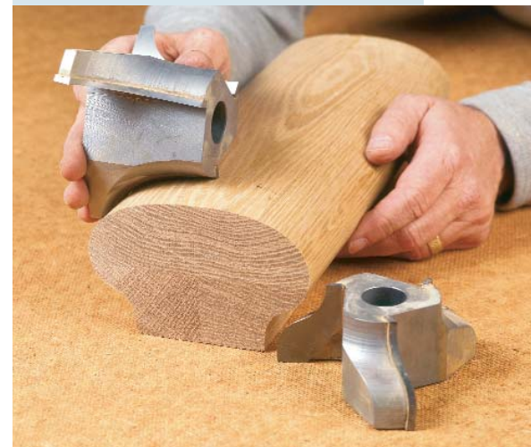
Custom-made, carbide-tipped wing cutters save time. Two cutters mold this large banister profile with the fewest setups.
