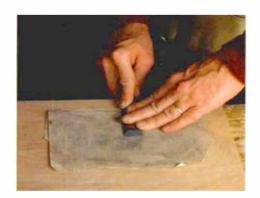
Remove the burr by rubbing the back of the tool on 120-gritpaper. Keep the tool perfectly flat on the paper.
