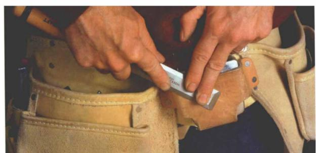
Atrop the bevel and back several times on any convenient piece of leather—a nail apron's tape holder, a belt or a work boot will do fine. Now you're ready to plane or pare.
