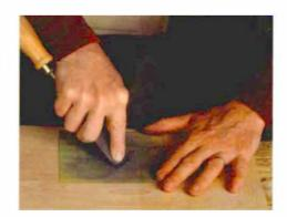
Continue honing with 60- and then 30-micron Microfinishing film. Remove the burr with the same grit.
