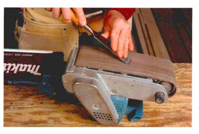
Grind the bevel. A 120-grit belt is usually as coarse as you'll need, but if there's a deep nick in the edge, go to 50-grit and then to 120-grit. Use a light touch, and don't let the chisel or plane iron stay on the belt for more than a few seconds at a time. If the tool becomes too hot to hold, it could lose its hardness. Let it cool before doing any further grinding.
