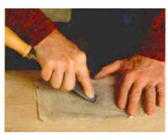
Use 120-grit on the bevel When the bevel has a consistent polish, flip the tool over, and remove the burr again.
