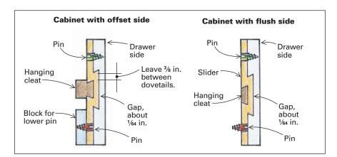
reach full extension, the bottom pin hits the back of the bottom slot, preventing the drawer from opening farther. The drawer is cantilevered from the slider and can't come out of the cabinet until the upper pin is removed.
