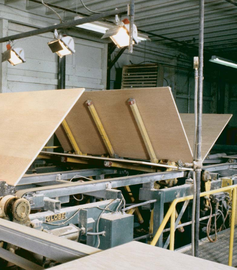
Final grading at the sanding station at a Columbia Forest Products plant in Klamath Falls, Ore. The birch panels on this machine, called a star grader, will soon be bundled and shipped.
