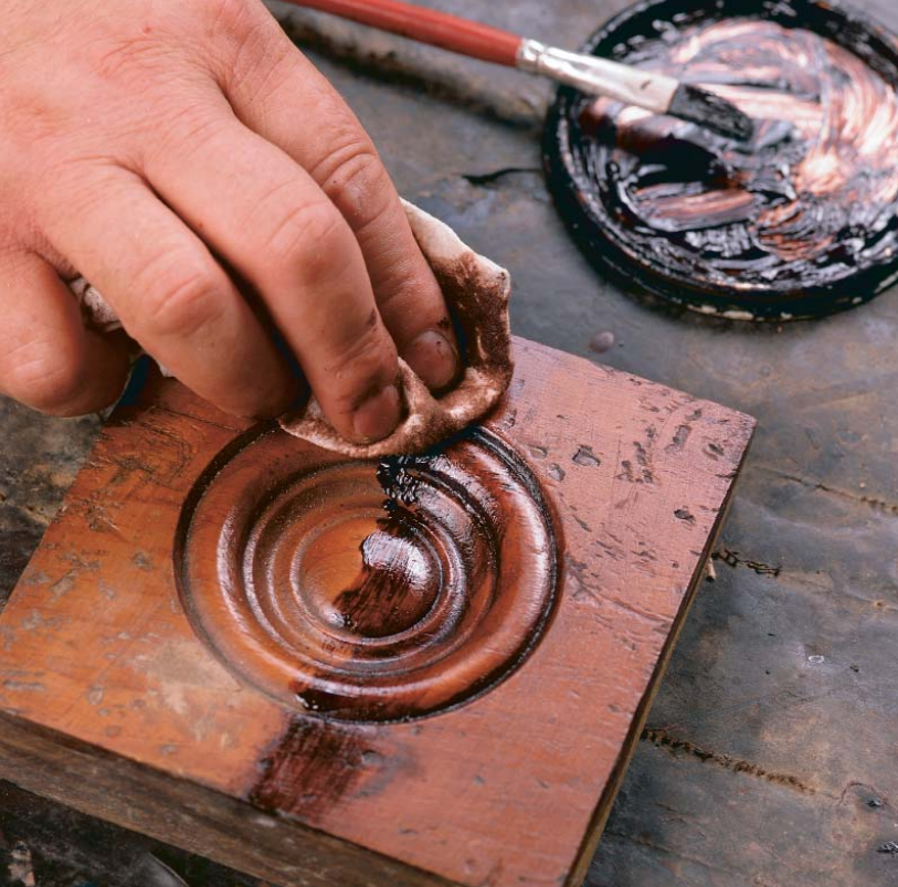
A glaze patina —The author applies dark glaze to a corner block for an old door frame to emphasize its age. After a light wash coat, he can dab on heavier coats in the recesses of the rosette and nail holes to simulate an accumulation of dirt.
