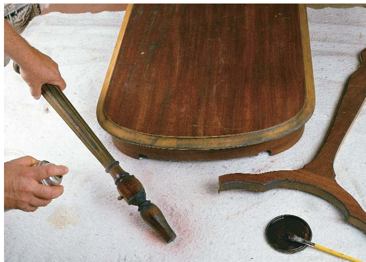
Toning unifies an antique sofa table. The author often tones and glazes furniture parts separately. Here, he sprays the legs and stripped table edge with a red mahogany toner. He used pigment from a can of dark stain to glaze the edges of the stretcher. The legs were wiped with this glaze, left to dry and then shellacked.
