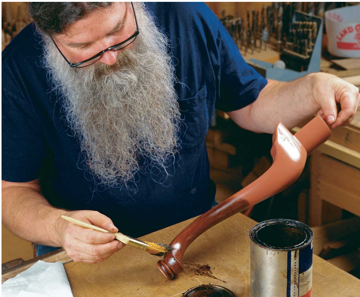
Glazing transforms color and adds detail. Glazes are colored finish layers applied over a sealed base, like this painted cabriole leg. Glazes stay workable long enough for blending and texturing.
