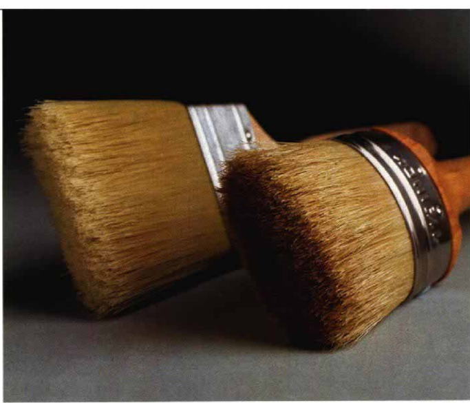
Same width, more bristles. The oval chisel-edge brush (right) will hold more finish than the flat chisel-edge brush. This allows varnish to be applied in long, smooth strokes.
