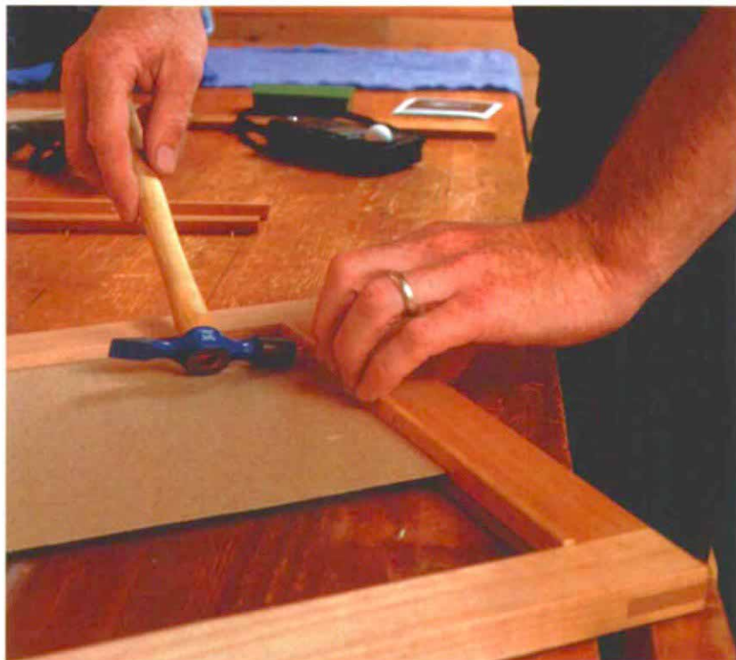
Protect the glass with cardboard, and carefully use a light hammer when setting the escutcheon pins.
