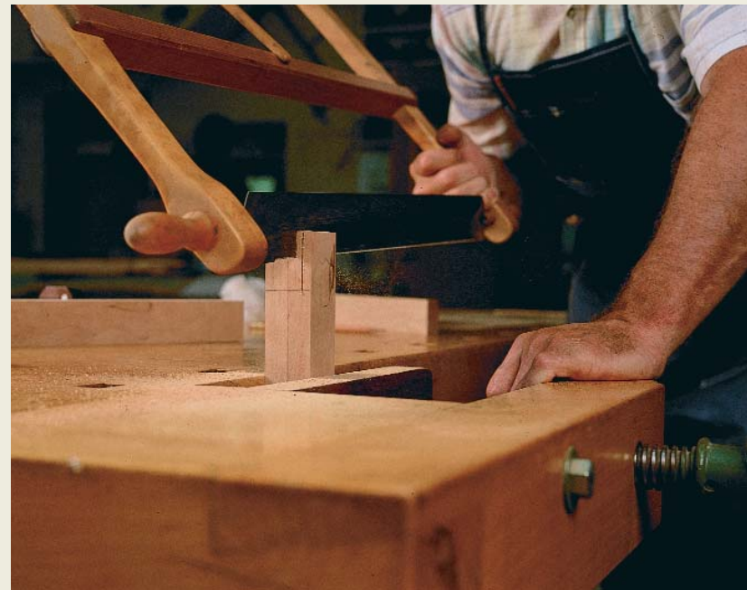
The bowsaw is Klausz's tool of choice for cutting this joint by hand because the long, wide blade tracks well and cuts quickly.
