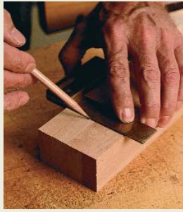
Mark the shoulder line. All pieces cut by hand must be marked on every side and end.
