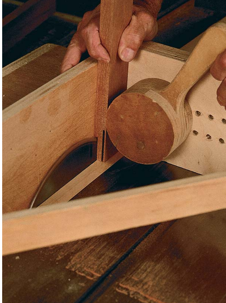
Cheek cuts for the tenon —To test the tenon setup, cut the cheeks first. The height of the sawblade off the table does not change. One pass per side is sufficient.
