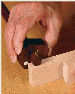
Mark mortises and tenons at the same setting. Fill in the scribed lines with pencil marks, so the lines are easier to read.
