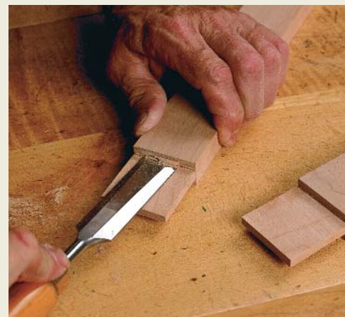
Fine-tune the fit. Rasps and chisels are good choices for removing material from either the tenon or the mortise. Hand-cut frames need many test runs before you can call them done.
