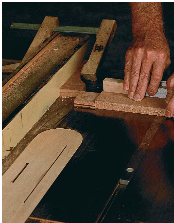
Shoulder cuts for the tenons are best done with a miter gauge. A scrap clamped to the fence acts as a stop. Self-stick aluminum carbide sandpaper on the miter gauge keeps stock from slipping.
