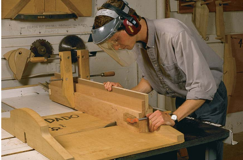
Mortises on the table saw —The tabletop mortises are cut with a dado blade and a cross-cut sled. Mating boards are clamped face to face against the sled's fence.
