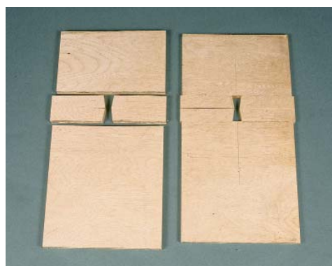
Butterfly-mortise jig , made of plywood, is cut to shape and glued back together.
