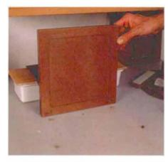
Tray with a cleat makes a good shortterm or job-site sharpening station. The author uses a scrapwood tray with a cleat that can be clamped in a vise.
