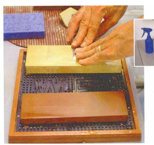
A dedicated sharpening station makes sharpening less of a chore. The convenience of having an area specifically for sharpening will take much of the hassle out of the process. And it doesn't have to be pretty: Scrap materials work just fine.
