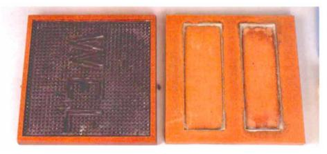
Trays keep stones from sliding around when you're sharpening. The old tray, on the right, is still in service and working fine after a dozen years. Water damage is just beginning to occur. The new tray uses a rubber mat to keep the stones from sliding around. The tray is kept in place with indexing pins set into the table.
