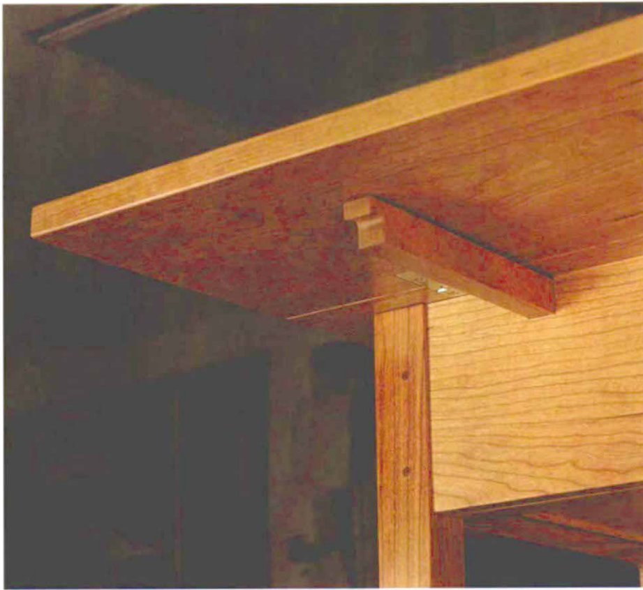
A sliding drop-leaf support is a neat, clean installation. It provides firm support that won't sag with use. The \frac{3}{8} -in.-long finger pull at the support's end is all that protrudes when fully retracted.
