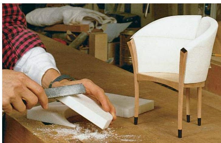
Cushion that's really foam—High-density, white polyurethane foam shapes easily and is perfect to mimic upholstery in scale models.
