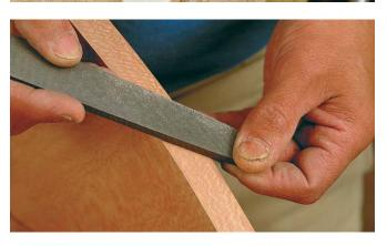
Chamfer adds a finishing touch-Using a smooth file (above), the author bevels the veneer edges, which eases and protects the table's corners and helps to disguise the seams.
