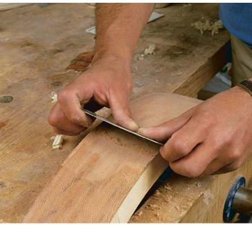
Scraping the veneer leaves a clean, smooth surface. Once the glue is cured and the veneer is set, the author uses a scraper to remove skid and scorch marks left by the iron. He keeps the scraper even and the strokes light to prevent the burr from digging into the surface.
