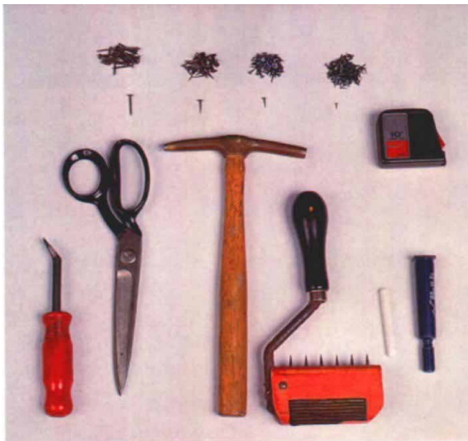
Basic upholstery tools for making a slip seat include from left to right: a tack lifter, shears, tack hammer and a webbing stretcher. You will also need webbing nails, no. 8, no. 3 and no. 2 upholstery tacks, chalk, a dark marker and a measuring tape.
