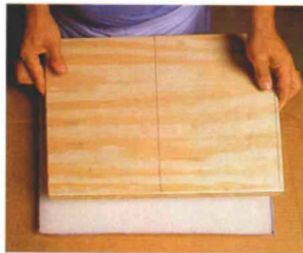
The extra cushioning provided by foam makes it practical and comfortable to build a slip-seat base by simply gluing high-density foam to a piece of \frac{1}{2} -in. plywood, which is then upholstered the same way as the traditional horse-hair slip seat.
