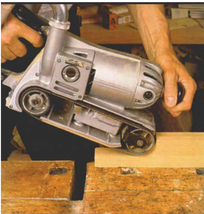
It takes practice to handle a belt sander with enough precision to smooth small-radius, curved surfaces with the front roller, as Becksvoort is doing here.
