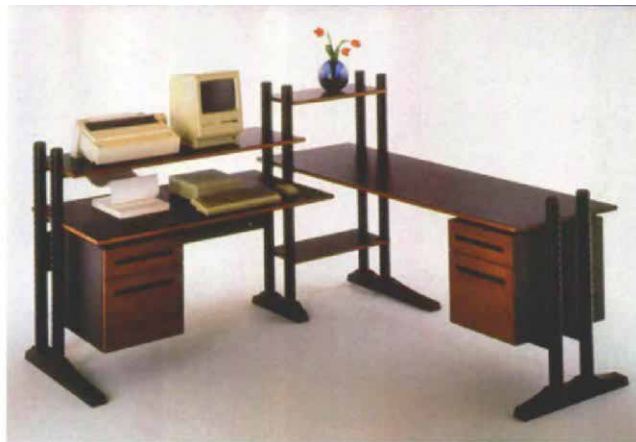
Dean Santner uses mahogany lumbercore plywood covered with plastic laminate for the surfaces and shelves in his "Motus" modular furniture system. The leg columns, which are painted with a tough acrylic finish, allow the height of each work surface to be adjusted independently for user comfort.
