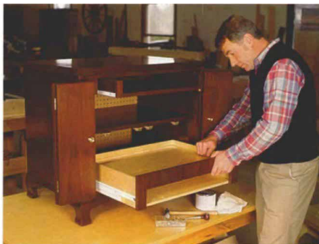
Frank Klausz does the final drawer adjustment on a computer cabinet he designed for an executive's office. The mahogany cabinet has bi-fold doors that conceal a pull-out keyboard and a two-tier printer drawer that has one slot at the front for loading paper, and another slot at the rear for paper to feed up to the printer.
