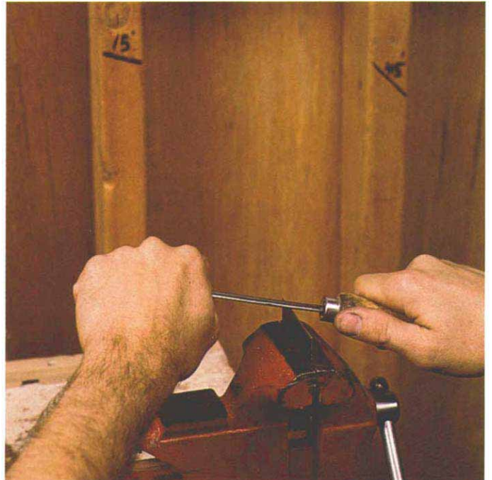
The final step in tuning the scraper is to form the cutting hook on the edge of the blade. The author is shown here burnishing the scraper's edge using a 15° line marked on the wall as a guide. Earlier, in preparation for forming the hook, the blade is flattened and its edge is made straight and filed to form a 45° bevel.
