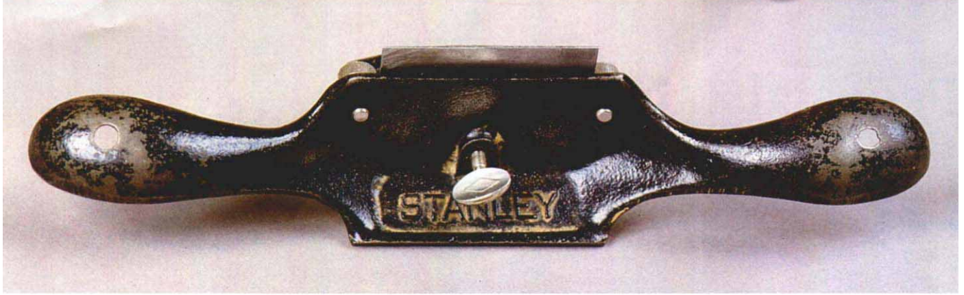
The cabinet scraper used by the author is a Stanley No. 80. For a newly purchased tool, it's necessary to flatten and polish the sole and modify the scraping blade to produce the best smoothing results. A carefully tuned tool will produce a surface ready for finish-sanding.
