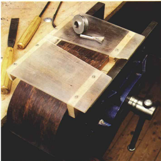
To rout the dovetail socket for the neck, the author uses a standard dovetail bit with a plastic template and a guide bushing.
