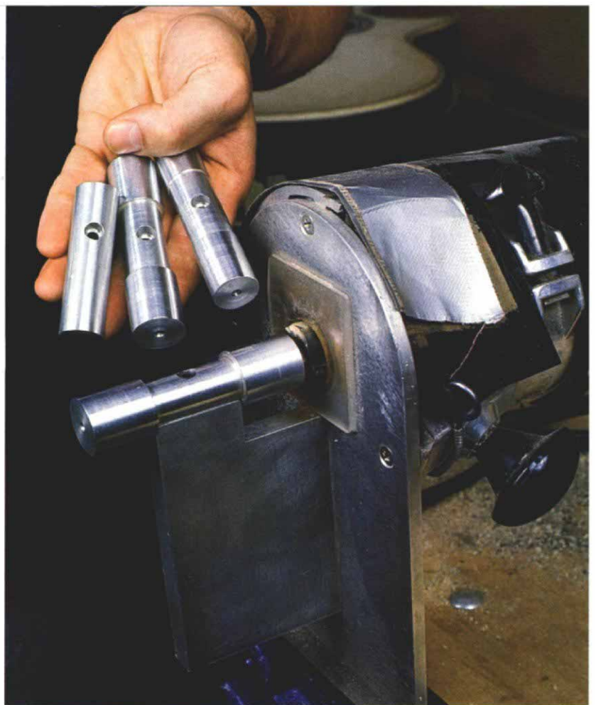
To rout the different-size grooves around the edges of the guitar for inlaying binding and purfling strips, Laskin made this routerjig. The side of the guitar bears on the turned aluminum rod as the instrument is moved through the cutter, while the front or the back of the instrument is pressed against the router base. Various rods control the width of the cuts; the depth is controlled by the router's own depth-setting adjustment. The tapered top edge of the smallpad in the center of the base allows clearance for the curved back of the guitar. A duct-tape shield directs dust down and away from the operator.
