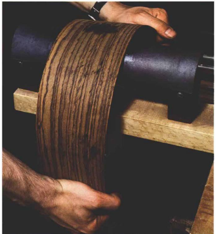
Guitarmakers shape the sides to conform to the guitar mold by bending the dampened wood over a heated pipe, moving the wood constantly to avoid kinks and scorching. With a little practice, the mold can be matched exactly.
