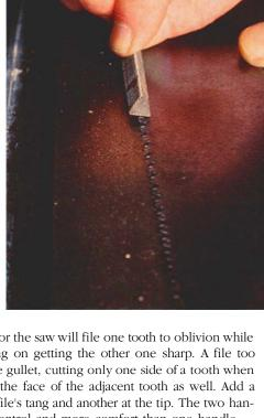
one that is too large for the saw will file one tooth to oblivion while you are concentrating on getting the other one sharp. A file too small will rattle in the gullet, cutting only one side of a tooth when it should be cutting the face of the adjacent tooth as well. Add a wood handle to the file's tang and another at the tip. The two handles provide better control and more comfort than one handle.
