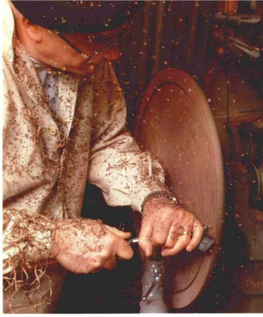
**4.** I turn the cove with a carbide-tipped scraper (soldered up for me by my favorite local machine shop) that has a profile like a flat little fingernail. This narrow profile allows me to fine-tune the shape of the cove until it exactly matches the profile of the gouge I'll use for the carving, as shown in the next step.
