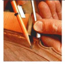
**12.** The next four photos show a critical part of the carving, extending the flat top up to the cove. Marking out is done with a compass, then stop cuts are made with chisels and gouges. Be careful not to make your stop cuts too deep, or they will mar the look of the top. The trick is to work the flat down gradually.
