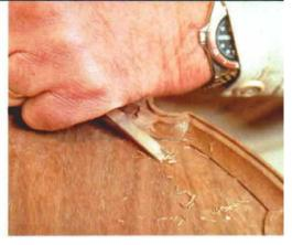
14. I've switched to a flat chisel here for paring away the gouge marks. Note the size of the chips and try to match them with your own tools. You must work in thousandths-of-an-inch—if you can't produce chips of this size, your chisel is dull. Check frequently with a small straightedge to be sure you don't go too deep.
