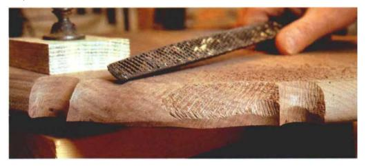
**16.** Here's the idea on the back. Rough out with a coarse rasp, then finish up with everfiner rasps and files until the wood shimmers. You'll probably find that the back has warped as a result of the dish on the other side. This is no problem, because the surface ought to be planed flat anyway, when the glue block is removed.
