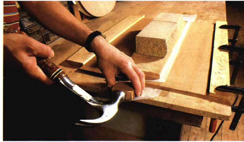
Guitar tops, as well as backs, are usually made of two pieces book-matched along a centerline joint. The joint can be glued by tapering the pieces, then gently tapping them into a matching pair of cleats that are fixed to the bench to form a wedge-shaped recess. A weight prevents the wood from buckling upward.
