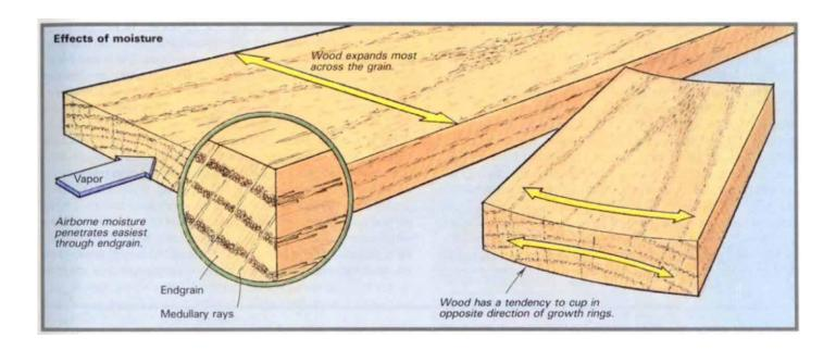
hether indoors and protected from weather, or outdoors and exposed to the elements, wood is always affected by moisture. It swells when it adsorbs liquid from rain, dew or moisture vapor in the air and shrinks as it dries.
